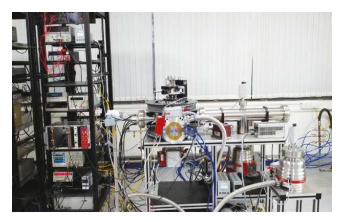
Experimental setup for absolute dissociative electron attachment cross section measurements in electron collisions with gas phase molecules of interest
