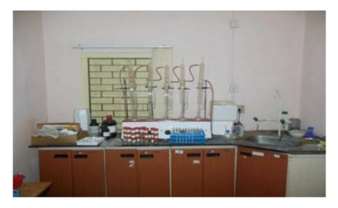
Reflux set up for Nitrogen Estimation via Kjeldhal setup
